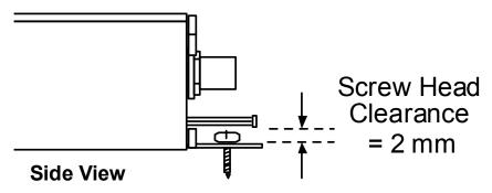
For example, one might use two 6-32 self-tapping screws 5/8" in length to mount the unit in a truck to the wall of the cab behind the passenger's seat.
